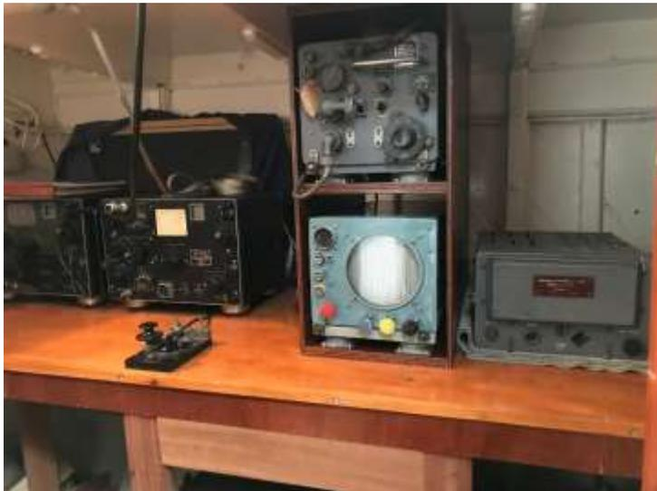
*TCS transmitter and receiver, type 286 radar and IFF unit in the wireless office.*
